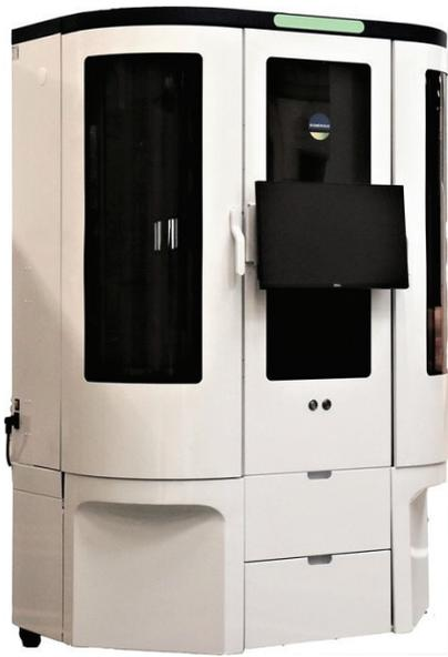
**Figure 2. 3P® STATION automated incubation and colony counting system.**
